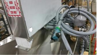
For shipping purposes, the connection to the start switch is removed, coiled and tied to the top of the machine.
