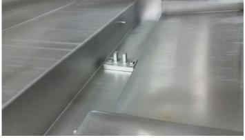
Rubbing block (285-6187) bolted in place
