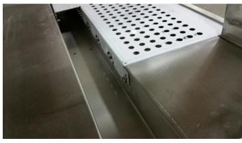
Ramp over the conveyor bar trough
