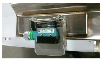
Switch bolted to shuttle and installed on tilt plate
