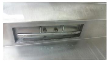
Bumper attached thru pocket to tilt plate
